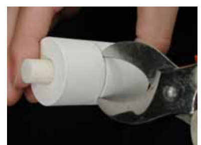
Fig.38 Final removal with a plaster nipper
