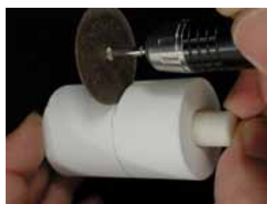
Fig.37 Section with a separating disk
