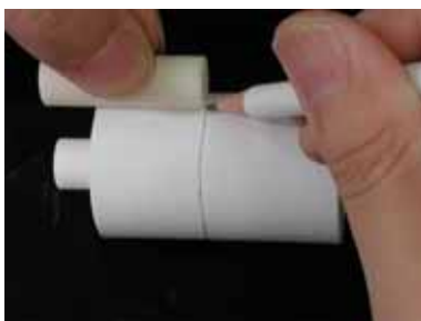
Fig.36 Marking the top position of the plunger
