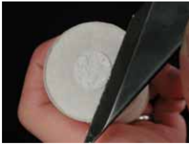
Fig.30 Remove the button of investment created by leveling cap
